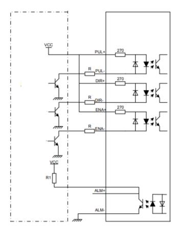
VCC is compatible with 5V or 24V; R(3~5K) must be connected to control signal terminal.
