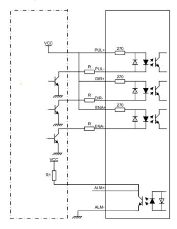
VCC is compatible with 5V or 24V;  $R(3^{\circ}5K)$  must be connected to control signal terminal.
