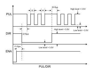
t1: ENA must be ahead of DIR by at least  $5\mu s$ . Usually, ENA+ and ENA- are NC (not connected).
